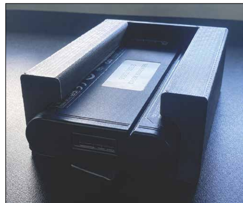
Figure 3. Battery installed in the printed mount.
