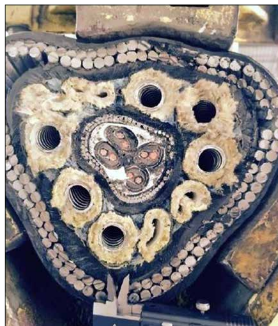
Figure 5. Umbilical cross section compressed in the experimental crushing test at 80 tf/m per shoe.
