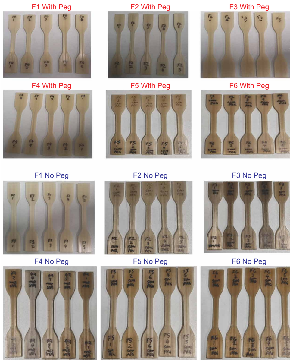
Figure 2. Tensile test specimen of composites obtained by 3D printing.
