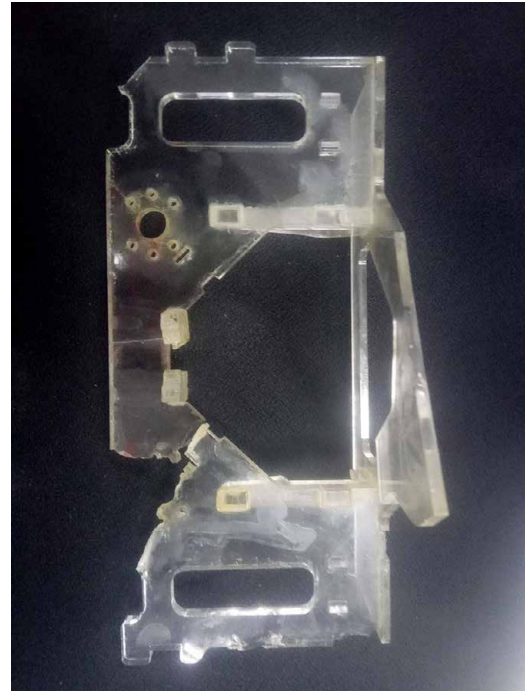
Figure 2. The acrylic structure supporting the thrusters was damaged.
