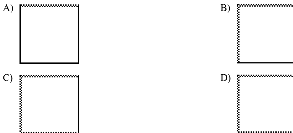
Figure 1. Square A with 1 perturbed side; square B with 2 perturbed sides; square C with 3 perturbed sides; square D with all sides perturbed.
