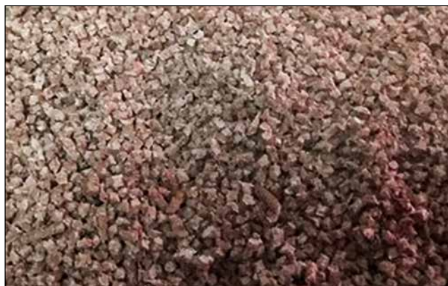
Figure 1. Masterbatch with 50% eucalyptus fiber.
