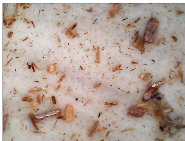
Figure 3. Optical microscopy of the composite with eucalyptus particles and HDPE matrix obtained from master-batch (image magnified 120x).
