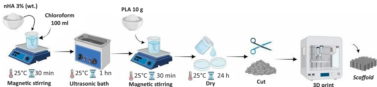
Figure 1. Composite scaffold manufacturing.
