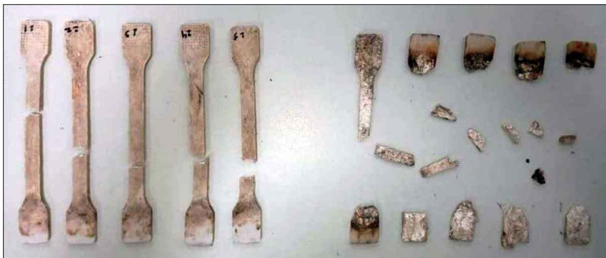
Figure 1. Test specimens after degradation and tensile testing (left: F0-S; right: F1-S).
