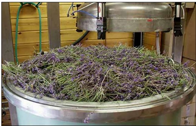
Figure 4. Typical steam distillation installation.
