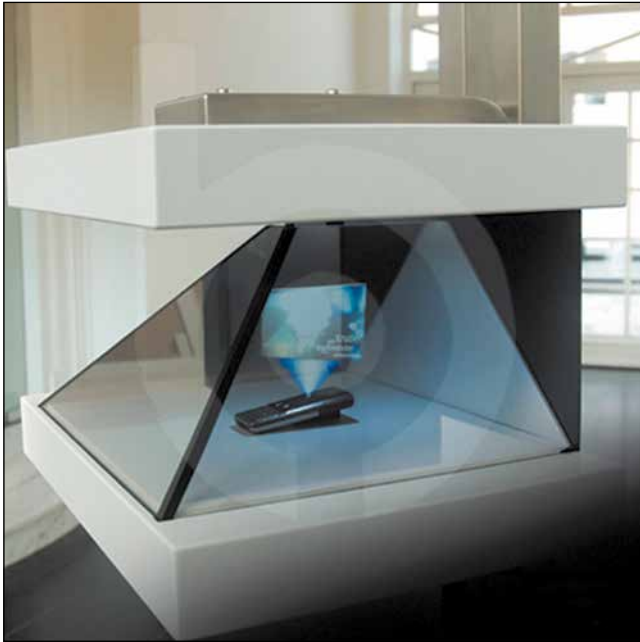
Figure 1. Three-sided holographic pyramid model with the overhead projector.
