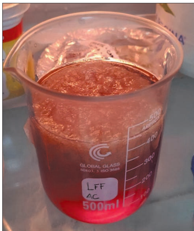
Figure 5. Precipitation of pectin with 96% ethanol.
