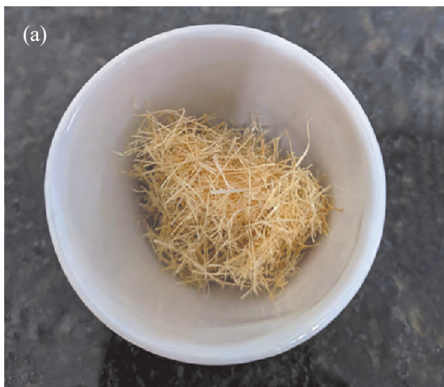
Figure 1. Fibers used. (a) sisal fiber; (b) PET fiber.
